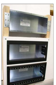
The *Adapter Plate* is attached to the *Back Box* through an opening in the sheetrock by (4) 6-32 Kep nuts. The mounting brackets, designed into each *Adapter Plate*, have enough adjustment to accommodate up to (2) layers of 5/8" sheetrock. After installation this provides a stable and ideal platform for the 16MU *Flush Mount Ring* to be attached. Shown to the left are the (3) stages of installation:
