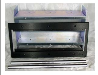
The **Back-Box** is comprised of a 11"(w) x 5"(h) x 3-1/2"(d) deep channel and 2 end plates for the mounting of the assembly to a single or multiple studs in a 4" thick wall. The channel has 3 concentric knockouts (1" + 1-1/4") in the top and bottom and one in each end plates for side entry when required.
