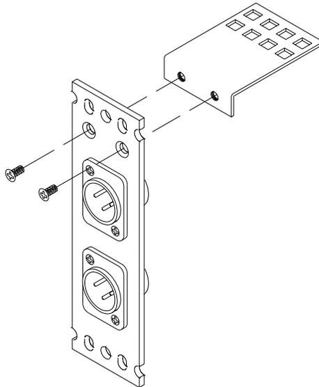
Using tie bars, panels may be grouped into "sub - panels", where a multi-conductor cable breaks out across multiple panels. Panel grouping is handy when combining panels for multi-channel applications. For example, we often provide tie line groupings of 8 channels to a location, with multiple appearances, say on both Elco and XLR. So, we would use 2 C3 panels (for the XLR's) and one B10 panel (for the
