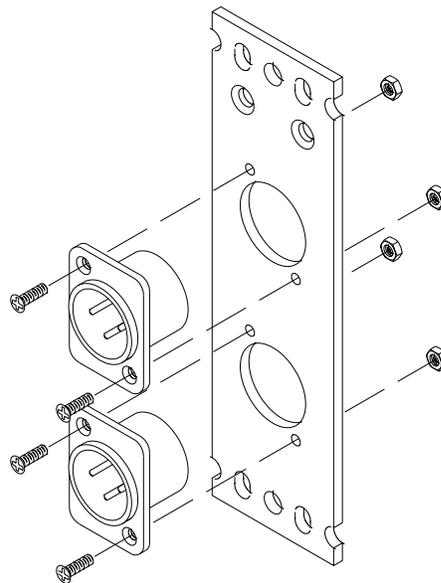
*Illustration of a MPS-B7-CM with knip nuts, standard panels are threaded*
