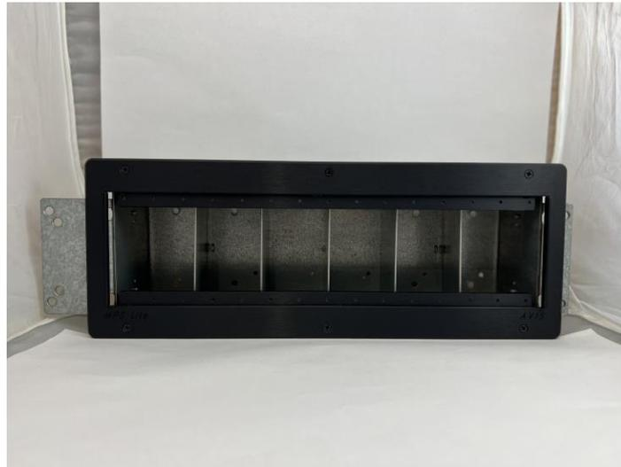
The **Adapter-Plate** is comprised of 2 parts, the first a formed aluminum plate that attached to the installed **back-box** via 6 screws and covers the cutout made in the sheetrock resulting in a low profile platform for the installation of our wide range of **MPS-Lite** modular panels.
