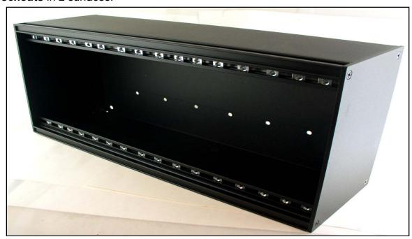
In the back we have a knockout for a 6-Gang Electrical Junction Box and in the bottom we have 2 Concentric knockouts for 2" and 1" conduit, plus a rectangular for Series 6000 Surface Raceway. To mount the enclosure to the wall we have 4 mounting holes in the back to make installation and connection to the enclosure easier and more flexible, with more options, for you.
