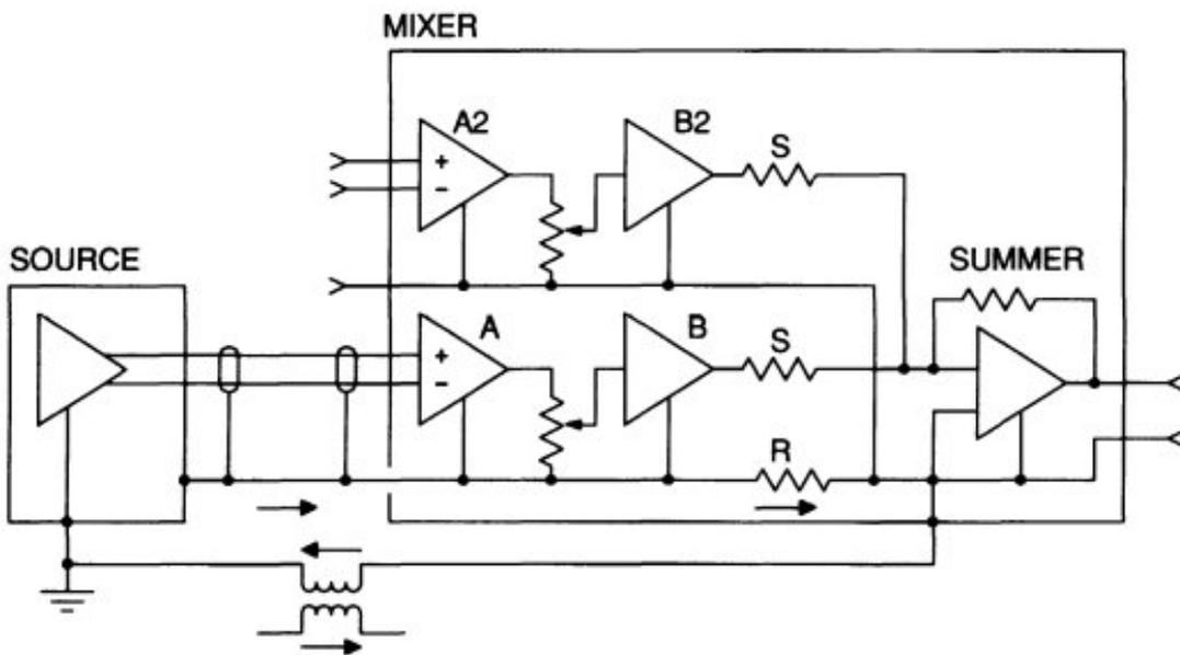
There is also a "reverse" pin 1 problem which has been documented in certain equipment. Due to proximity of ground traces or wiring to the power transformer inside the box the equipment itself is capable of inducing noise voltages between input and output jacks.
