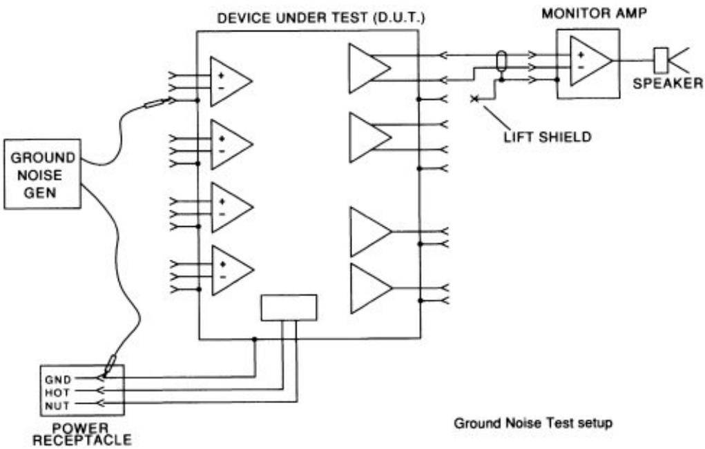
If you find a piece of equipment with a pin 1 problem, you might consider modifying it by re-routing the shield terminals directly to the chassis internally. Take care though - you may be voiding a warranty by doing this!
