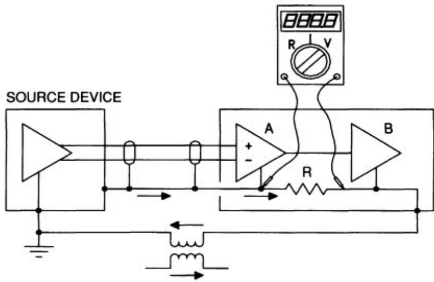
The pin 1 problem can be even more confusing than this. In the next example, the internal detection occurs in the summing stage of a mixer. Currents injected into an input shield are detected by trace resistance R. Even if the input fader is down the buss noise is elevated. This can be extremely confusing if you think that you have isolated an input by turning down it's fader!
