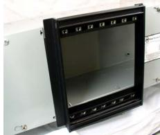
to the enclosure is straight forward, simply insert the head of supplied 6 -32 hex head machine screws into the dedicated slot located in the rear of the extrusion, then poke them through cover screw holes before tightening the knep nuts on the inside of the enclosure...... done.
